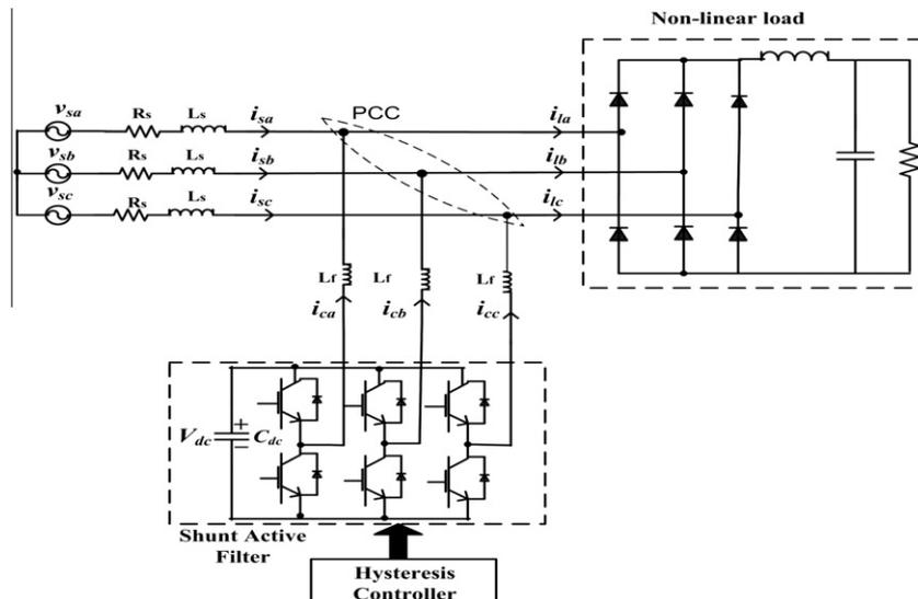
Fig. 1. System configuration with practical realization of SAF.
