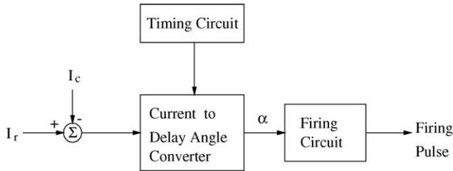
Fig. 2. Control scheme for the FC-TCR SVC.
