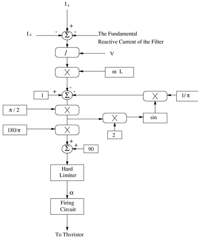
Fig. 3. Modeling of control system in EMTDC.
