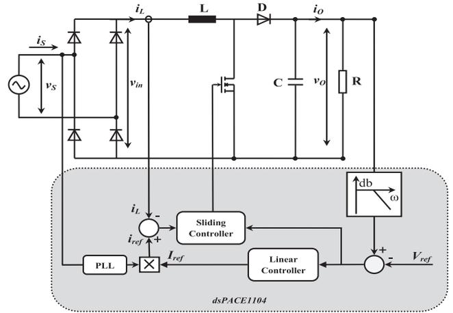
Fig. 2. Boost converter circuit governed by sliding mode controller.
