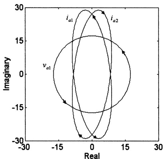
Fig. 2. Locus of instantaneous positive and negative sequence currents.
