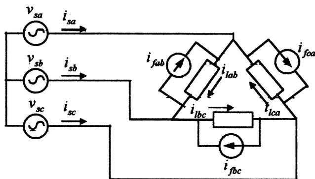
Fig. 1. Schematic diagram of the compensation scheme.
