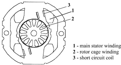
Fig. 1. Cross section of the shaded-pole motor.
