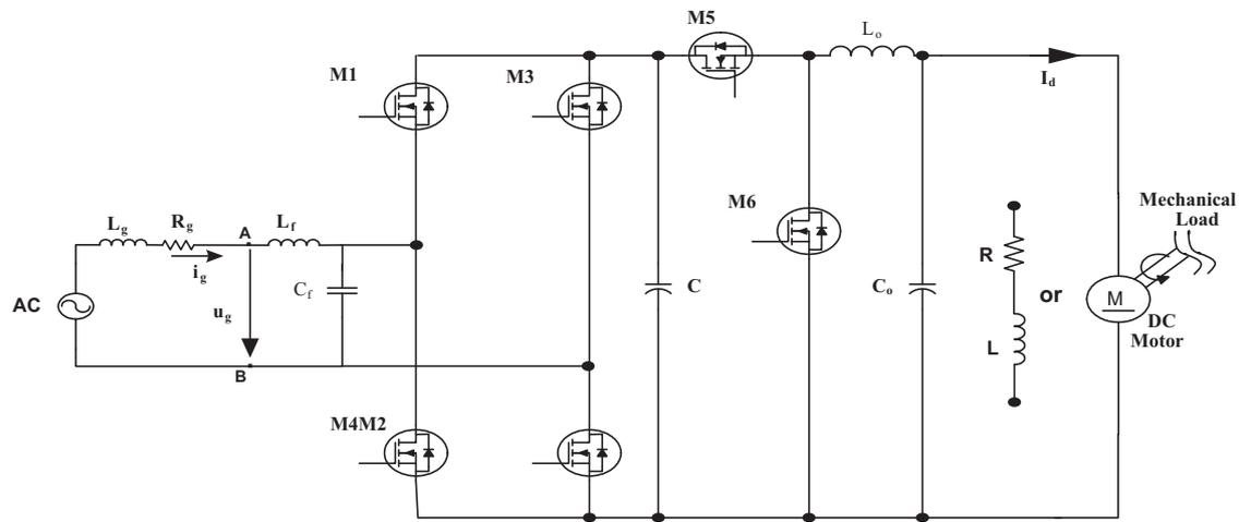
Fig. 1. Converter structure for bidirectional current flow.
