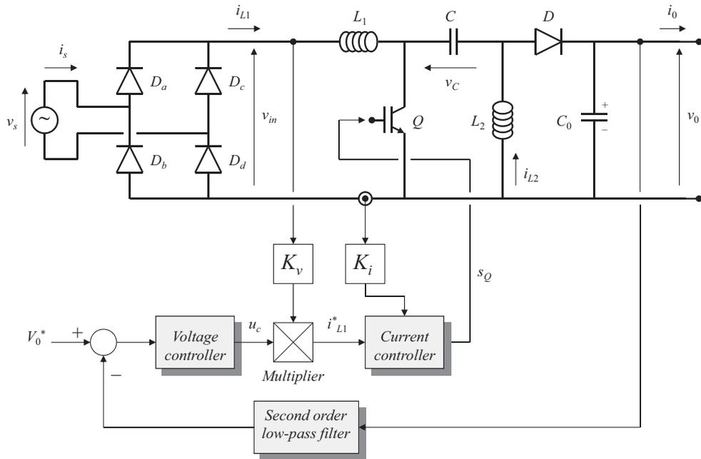
Fig. 1. Buck–Boost SEPIC power factor correction circuit and its control system.
