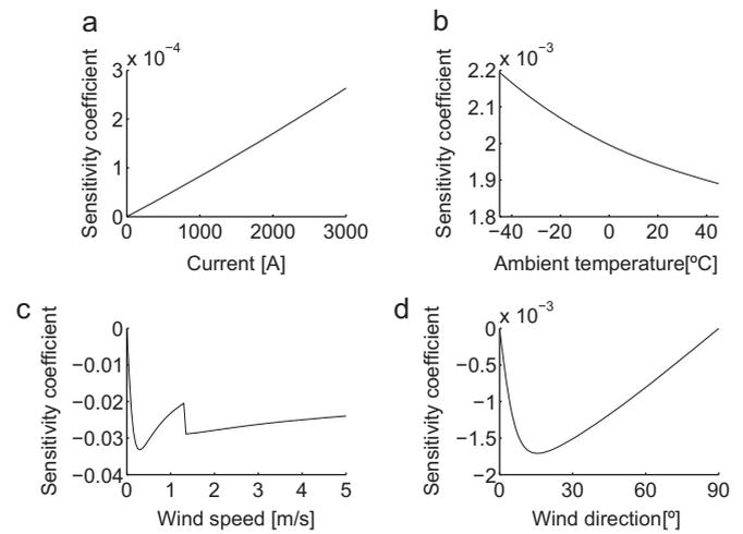
Fig. 1. Variation of sensitivity coefficients of the conductor temperature with respect to the electrical current (a), ambient temperature (b), wind speed (c), and wind direction (d). Parameters:  $T_c = 50.5$  °C,  $i = 1500$  A,  $S = 500$  W/m<sup>2</sup>,  $T_a = 0$  °C,  $v = 2.5$  m/s,  $\varphi = 45$ °.
