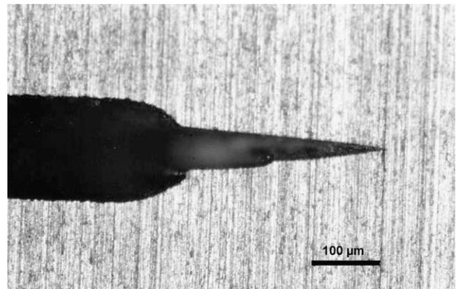
Fig. 2. Optical micrograph of a typical notch.
