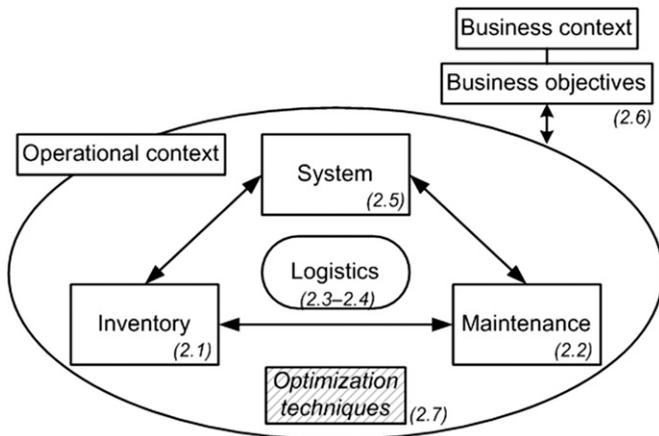
Fig. 1. Framework for joint maintenance and inventory optimization models.
