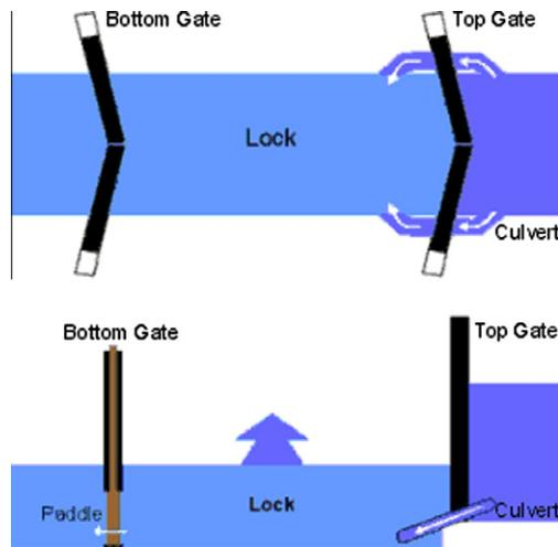
Fig. 1. Plan and side views of a lock.
