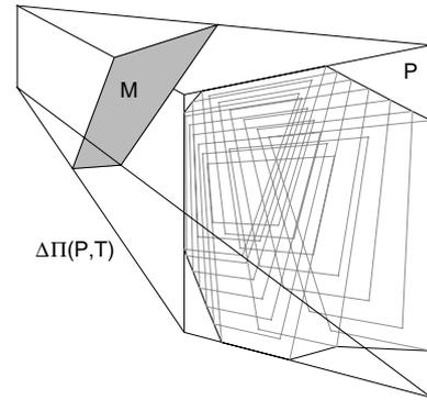
Fig. 3.  $M$  defined in the core of a sunlighting volume  $\Pi(P, T)$  has its shadows within  $P$  whatever the instant of  $T$  is.
