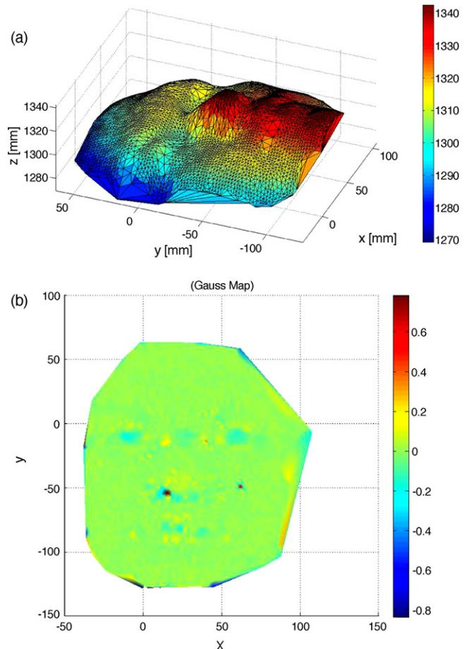
Fig. 2. (a) Geometrical representation of a scanned surface (the colour-map describes  $z$ -coordinate values [mm]); (b) curvature map for the same surface (the colour-map describes curvature  $K$  values).
