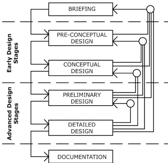
Fig. 1. The iterative design process.
