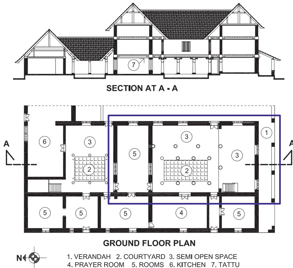
Fig. 1. Plan and section of *Puthiya Kovilakam* located at Nilambur – selected area is marked in rectangle [36].
