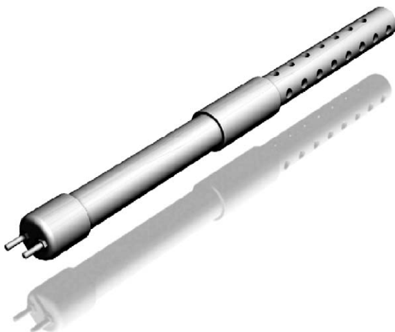
Fig. 1. Illustration of a typical wood-disc moisture probe (drawn by Neill Hughes).
