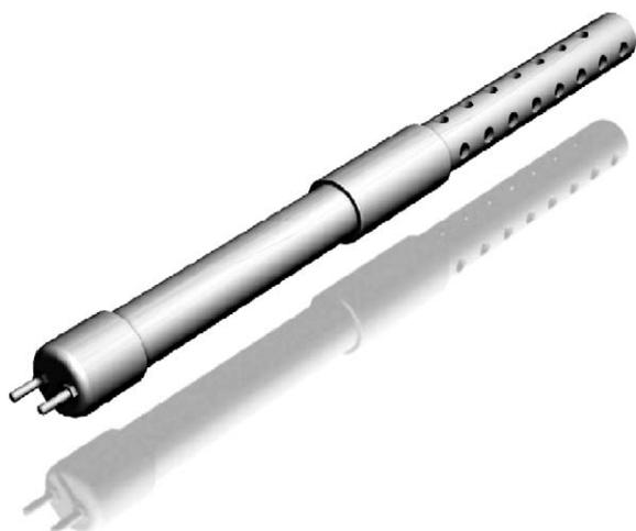
Fig. 1. Illustration of a typical wood-disc moisture probe (drawn by Neill Hughes).
