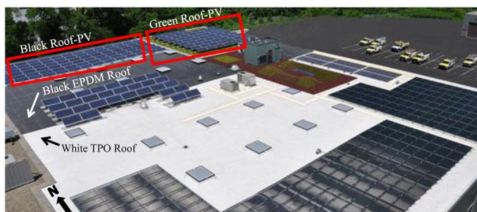
**Fig. 1.** Two designated study areas (black roof–PV and green roof–PV) on the Sunscape Demonstration Project [35] (For interpretation of the references to color in this figure legend, the reader is referred to the web version of the article.).
