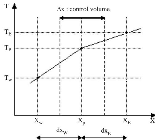
Fig. 1. Temperature distribution.
