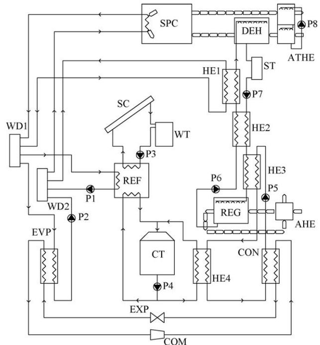
Fig. 1. Schematic diagram of hybrid air-conditioning system of green building.
