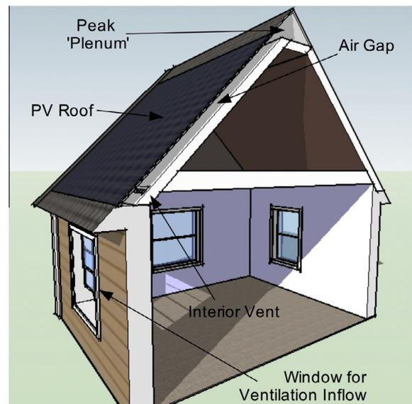
Fig. 1. Configuration of a ventilated roof.
