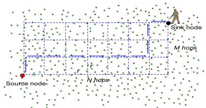
Fig. 1. Grid-based topology in wireless sensor network.
