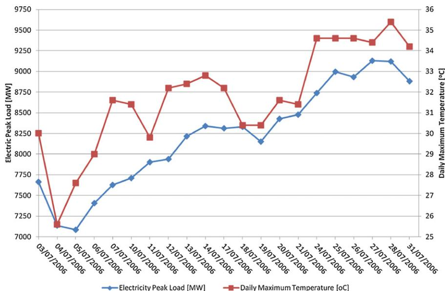
Fig. 2. Correlation between daily maximum outdoor temperature and daily maximum electricity load [3].
