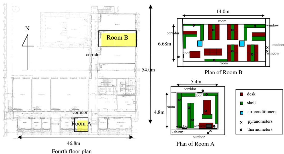
**Fig. 1** Floor plans and location of measuring apparatus.
