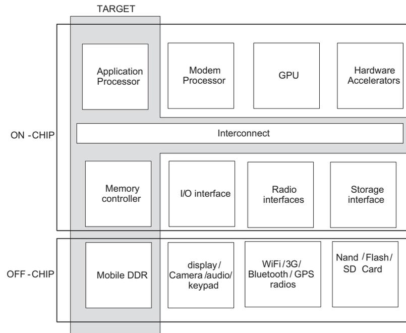
**Fig. 1.** High-level view of a mobile phone architecture.
