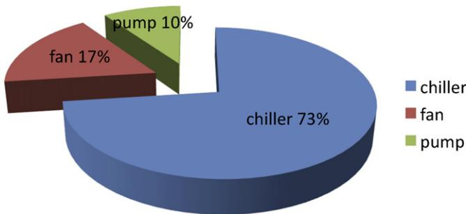
Fig. 2. Energy consumption of different components in a sample cooling session.
