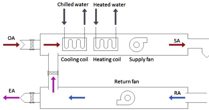
Fig. 1. Schematic diagram of a typical AHU system.
