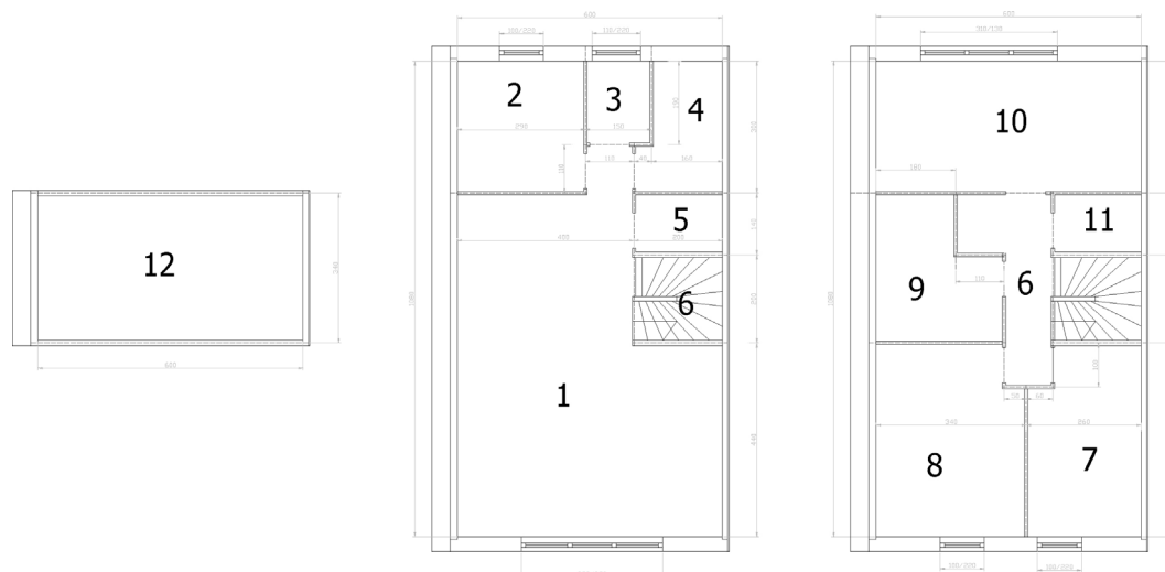
Fig. 1. Attic, ground and first floor plans and their zoning in the passive house of JDL type. 1 – living room; 2 – kitchen; 3 – vestibule; 4, 11 – utility room; 5 – WC; 6 – staircase and hall; 7, 8 – children's rooms; 9 – bathroom; 10 – bedroom; 12 – technical room, total living area 120.1 m 2 .
