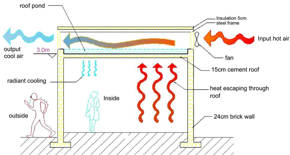
Fig. 2. Thermal performance of roof pond with forced electric ventilation.
