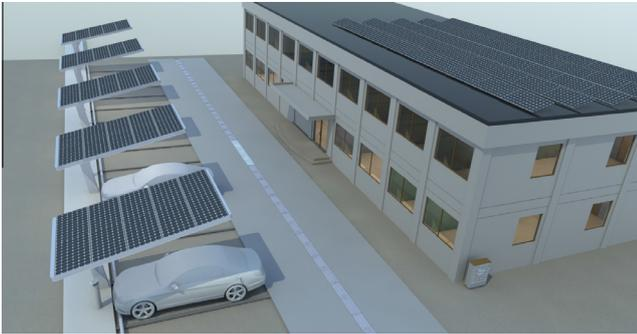
Fig. 1. Design of solar powered EV charging station.
