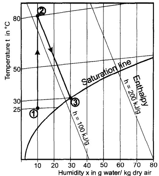
Fig. 1. Heating and humidifying process in h-x-diagram.
