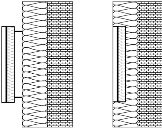
**Fig. 1.** Schematic drawings of a building-added solar thermal collector (BAST, left-hand side) and a building-integrated solar thermal collector (BIST, right-hand side). The solar thermal absorber is indicated by a thick black line, the masonry with a brick pattern and the insulation of the wall and of the collector with insulation battening patterns.
