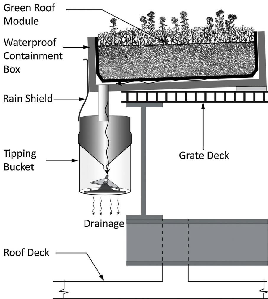
Fig. 1. Cross section of green roof module, waterproof containment box, rain shield, and tipping bucket.
