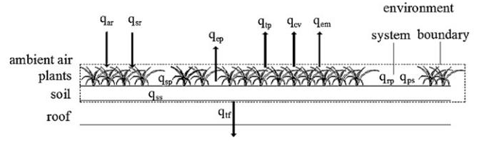
Fig. 1. Energy exchange between an extensive green roof and its environment.
