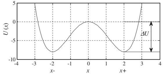
Fig. 1. The bistable potential function  $U(x)$ .
