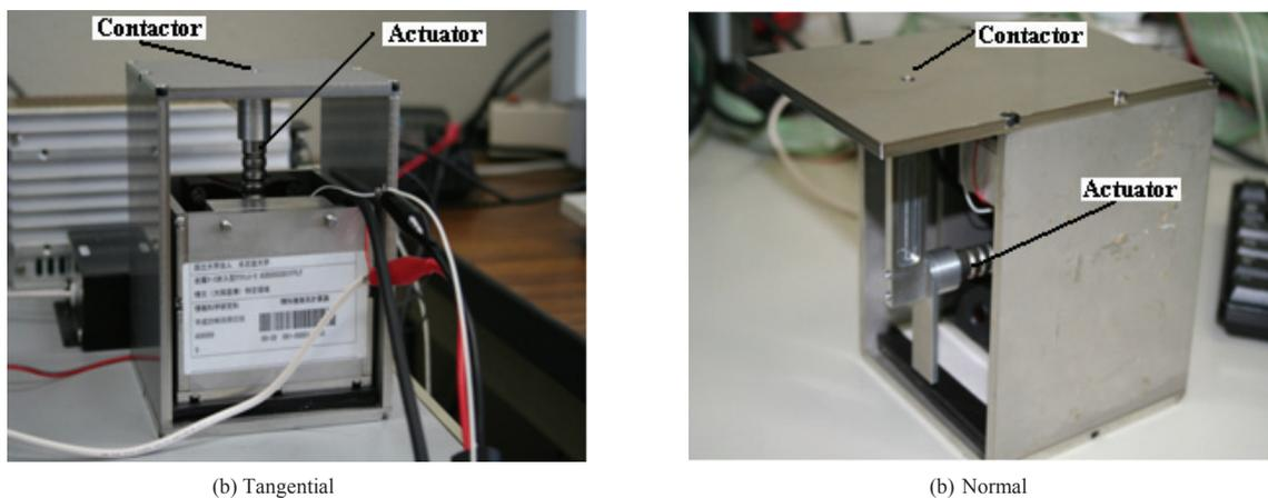
Fig. 1. Vibrating stimulation generator using piezoelectric actuator.
