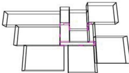
Fig. 1. Divided zone of assumed building for CFAST model.
