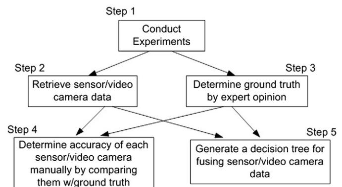
Fig. 1. Methodology for blockage assessment of buildings.
