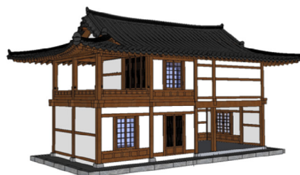
(c) A two storied specimen with ‘I’ shaped plan
