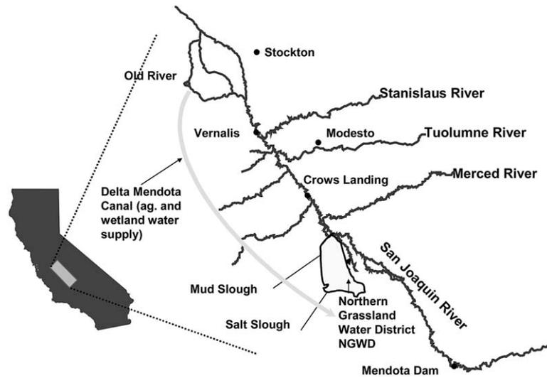
Fig. 1. SJR Basin showing NGWD and the major west-side wetland drainage conveyances Mud and Salt Sloughs. Water supply to agriculture and wetlands in the Grassland subbasin is provided through pumping from the Sacramento—San Joaquin Delta via the Delta Mendota Canal.
