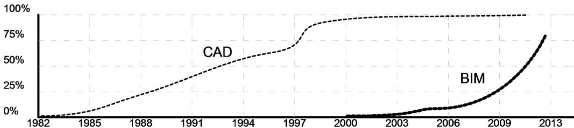
Fig. 2 The process of implementation of a new way of working in the UK / USA. BIM has been implemented here twice faster than CAD in its time [1].
