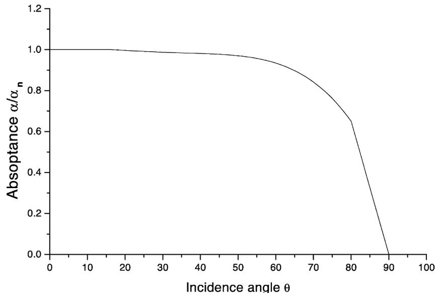
Fig. 1. Dependence of absorptance on incidence angle.
