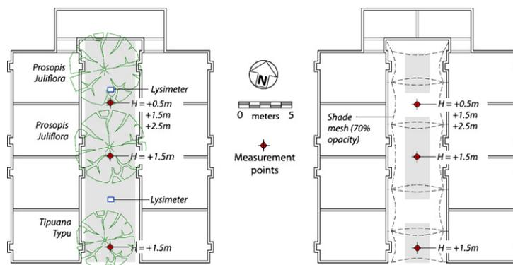
**Fig. 1.** Plan showing location of measurement points (in both courtyards), of trees in west courtyard (left) and of shading mesh in east courtyard (right). The grey area drawn for convenience only in west courtyard shows extent of grass cover in both courtyards, once it was applied. The grey areas shown in the east courtyard indicate the extent of bare soil in both courtyards; the rest of the ground surface was paved.
