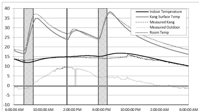
Fig. 2. Predicted and measured temperature profile on 11/24/2008.
