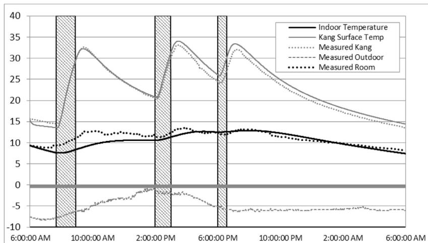
Fig. 1. Predicted and measured temperature profile on 2/19/2009.
