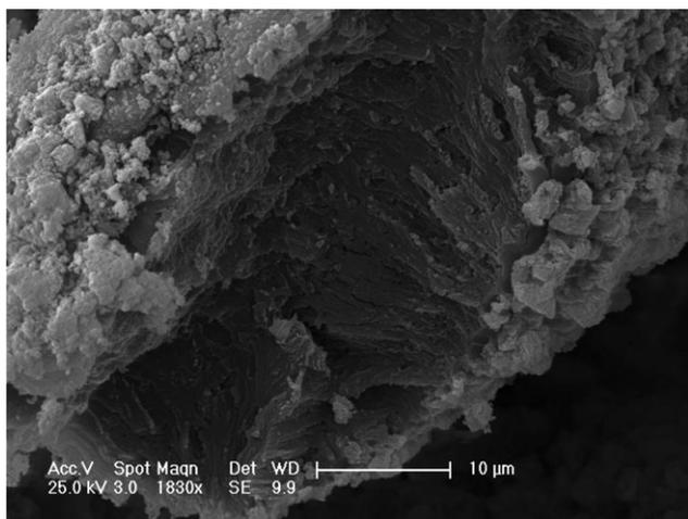
**Fig. 2.** Scanning electron microscope image of a void left in lime plaster following the dissolution of hair. The lining of the void mirrors the pattern of cuticle scales from horse hair. This sample formed part of a plaster frieze in Elcho Castle, Perthshire, Scotland.
