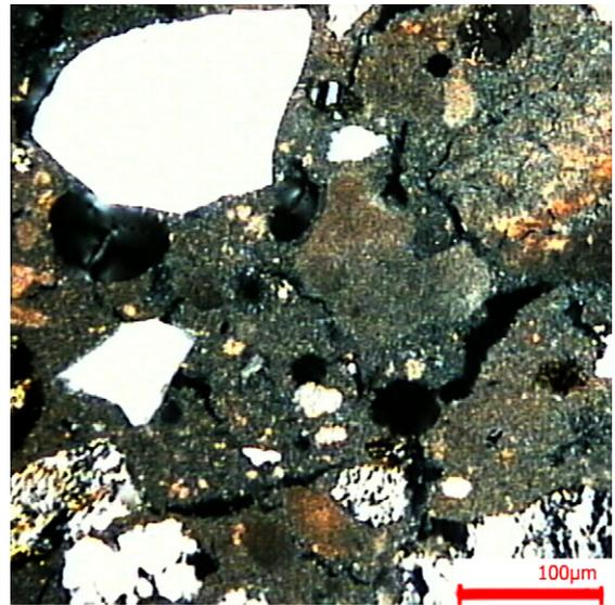
**Fig. 3.** Cracks and pores in the structure of a lime mortar from Bezesteni in Thessaloniki 15th century AD) (polarized microscope, author's archives).
