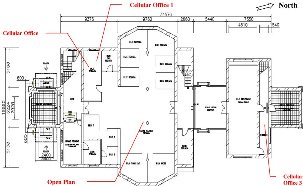
Fig. 1. Ground floor plan of the office building.
