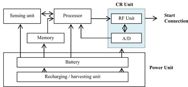
Fig. 1. Hardware structure of CRSN.
