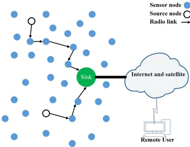
Fig. 1. Sensor nodes scattered across a sensor field.
