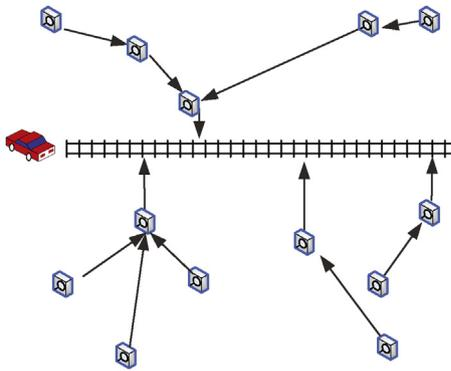
Fig. 1. Sensors transmit data to mobile sink by relaying in a multi-hop manner.
