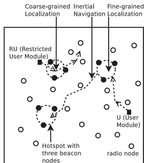
Fig. 1. User module  $U$  and restricted user module RU in a typical graded precision localization setup.
