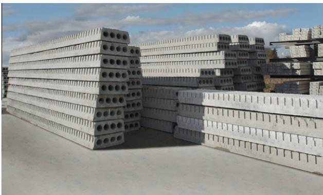
Fig. 1 Pre-stressed hollow core strip slab.
